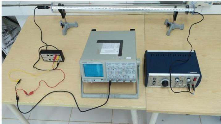
**Gambar 7.2.** Skema rangkaian pipa organa tertutup.
